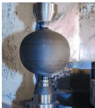
Figure 1 Taylor bowl being shaped by a lathe [6]
